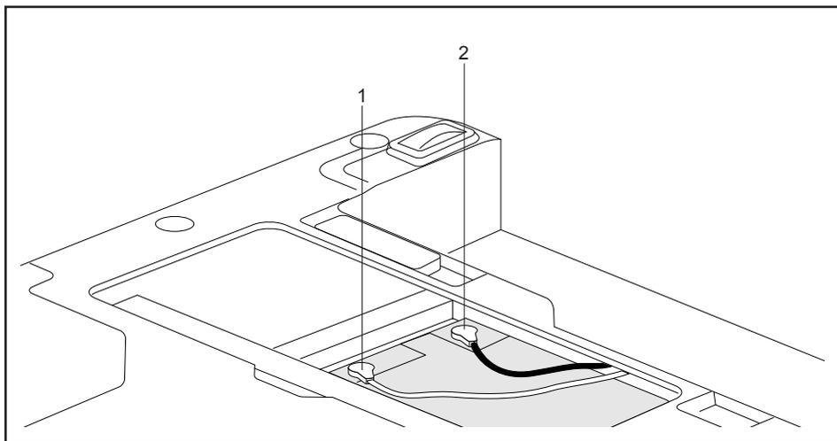
The dots indicate the positions for connecting the two antennas to the UMTS/LTE module (1: orange; 2: yellow).
